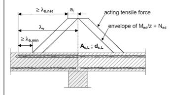
**Figure A2:** Overlap joint at a foundation of a column or wall where the rebars are stressed in tension
